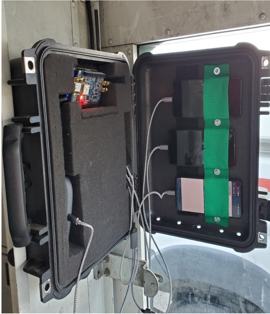
Figure 1. A completed kit, open to show the contents, as installed in a USPS model delivery vehicle. The three smartphones as mounted in the lid are level with the window and windshield for maximum signal penetration when the case is closed. The spectrum sensor is located at the top left with a red LED, with the MiFi for sensor data communication below that. Both are positioned in the foam interior. A single monopole RF antenna for the spectrum sensor is visible at the top, on the outside of the box. A small GPS antenna for the spectrum sensor is also mounted at the top but is not fully visible in this image. The power cables for the smartphones and MiFi are shown. These cables fit cleanly in the space between the smartphones and the interior foam when the lid is closed.
