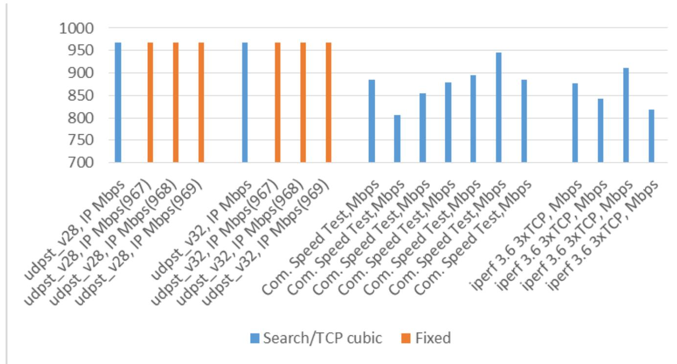
udpst, Common Speed Test Web Sockets Clients and iPerf 3.6 with TCP Cubic (default), in NJ
